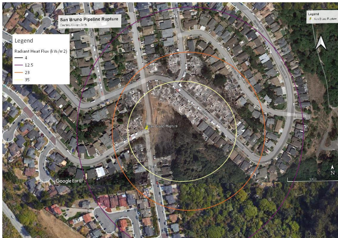
Figure 27 Radiant Heat Flux, San Bruno Pipeline Rupture and Fire
