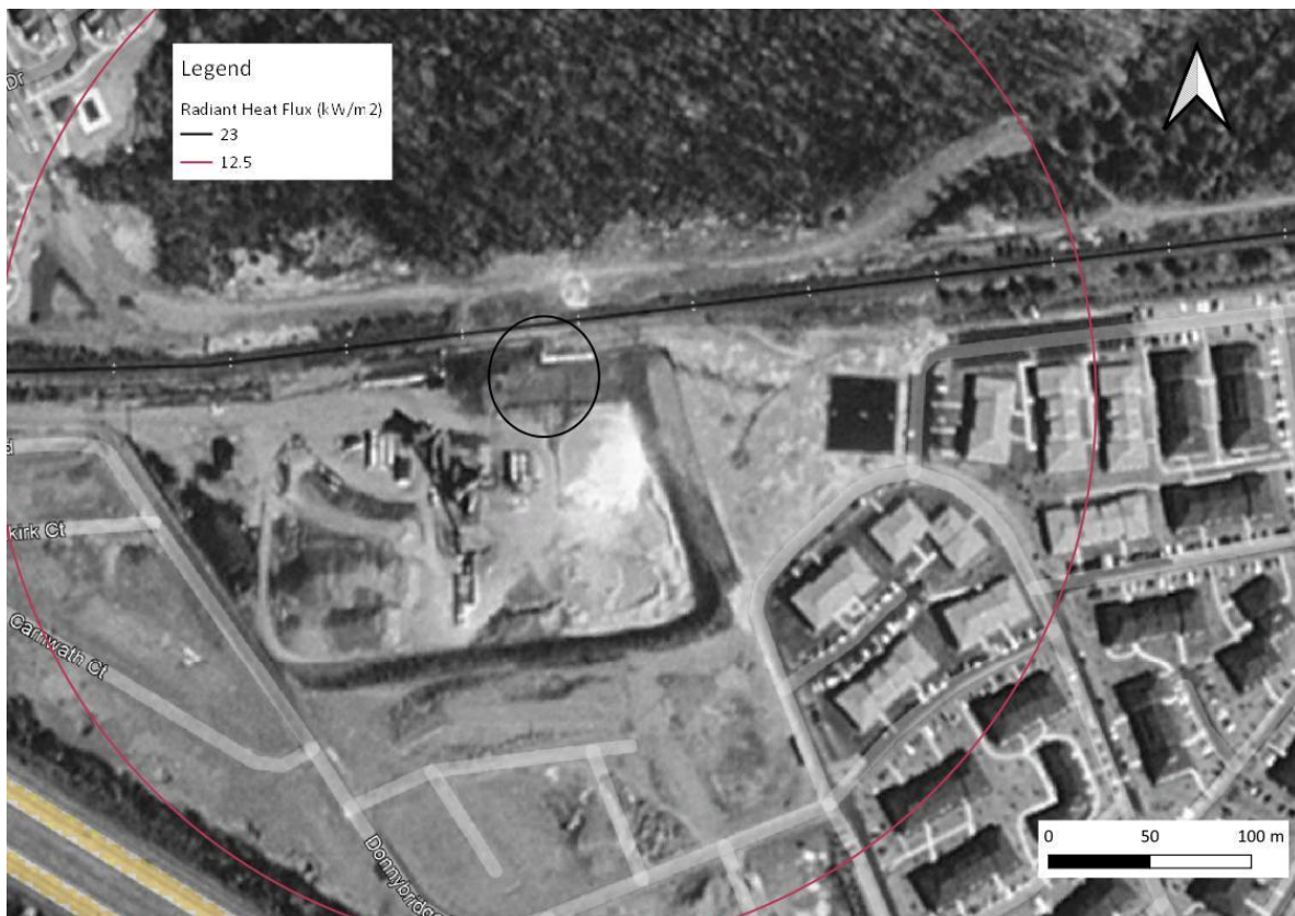
Figure 30 Radiant Heat Flux, Edison Pipeline Rupture and Fire
